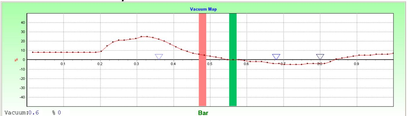
This is the main vacuum correction map. Use this map to adjust enrichment deviations for the specific engine. Also use this map on the left side to adjust idle mixtures for an automatic gearbox when selecting drive.
