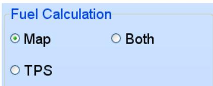
**Fuel Calculation** – This setting is to allow the tuner to choose Map sensor calculation or Throttle sensor calculation or a split of both signals.
