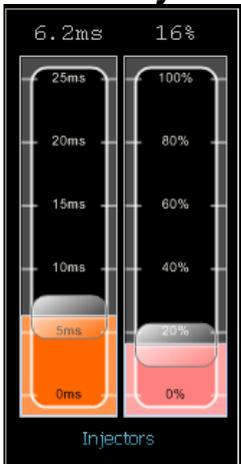
This ms bar indicates the time in milliseconds that the injectors are opened. For a 4-stroke engine this is measured over 2 revolutions and for a 2-stroke engine it is measured over 1 revolution.
