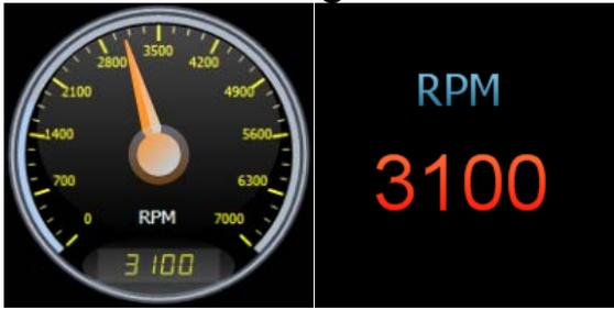
RPM - This is the current engine revolutions. Double click will toggle between the two options.
