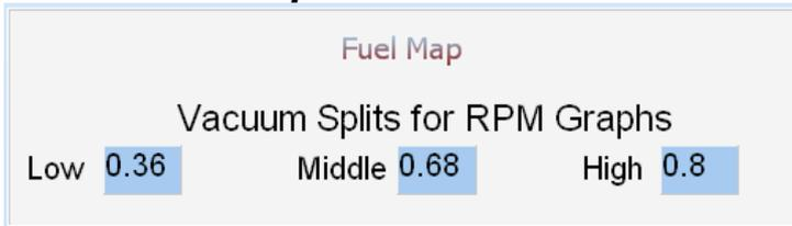
These limits are used to select between the four RPM fuel correction maps. They are displayed on the vacuum map as three blue arrows. When the vacuum signal passes these arrows, a different RPM correction map is used.
