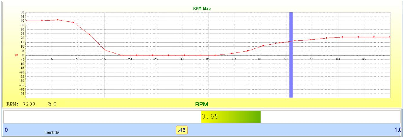
These two graphs will manipulate the target voltage with a certain percentage. This feature requires a 4 Wire Lambda sensor with element. It will not manipulate the fuel if the water temperature is below 60°C or if the startup delay time is not over.
