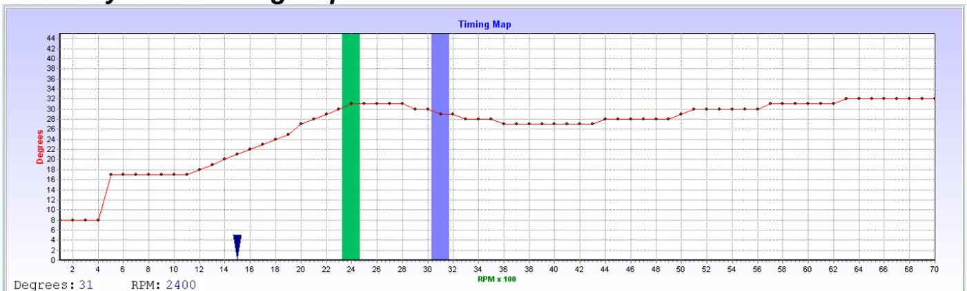
This Timing map is the wide open throttle map. Here you set the maximum timing of the engine trough the whole RPM range. If the engine ping or detonate, see at which RPM's it happens and bring the graph 3 to 4 degrees down at that RPM range.
