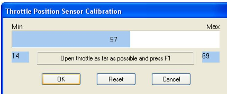
A screenshot of the 'Throttle Position Sensor Calibration' dialog box. It features a horizontal slider bar with 'Min' and 'Max' labels. The current value is 57. The range is from 14 to 69. A text box contains the instruction 'Open throttle as far as possible and press F1'. There are 'OK', 'Reset', and 'Cancel' buttons at the bottom.
