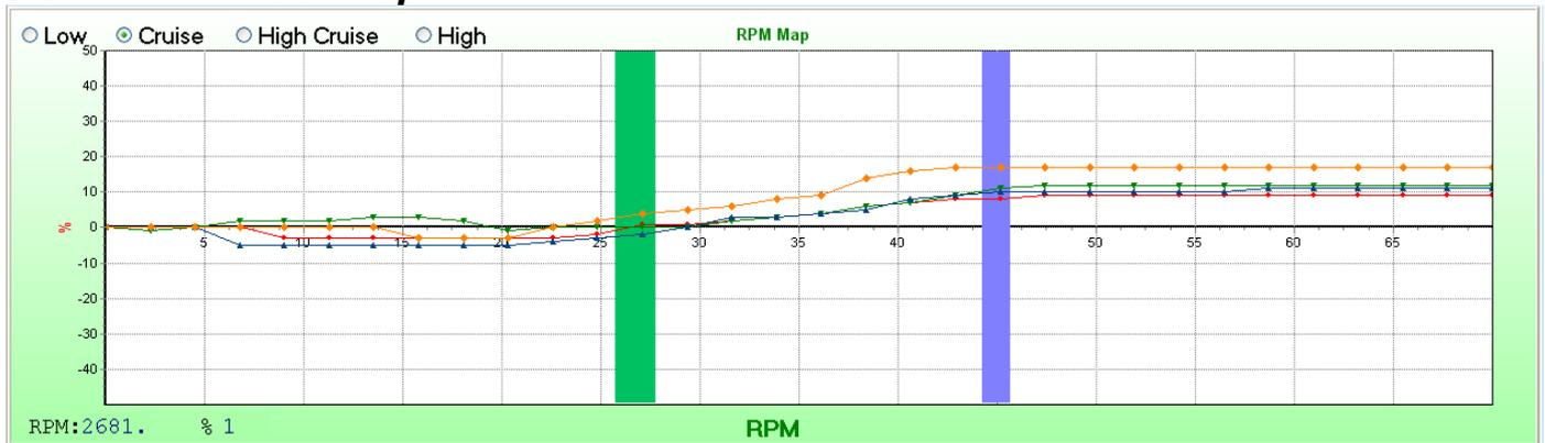
This graph is used to adjust enrichment in different vacuum zones. It is divided in four groups on the top graph with the Blue arrows. Select the Low, Cruise, High Cruise or High setting and adjust the fuel enrichment over the rpm range for the specific graph.
