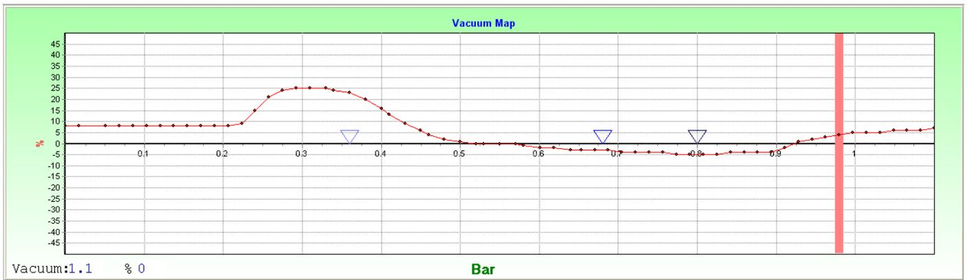
Now by adjusting the Dyno RPM's plot out the RPM fuel map. Again use the right air-fuel mix required for the different RPM's. Normally on this map you should be on the rich side. If you hear detonation or pinging go to the RPM timing map and retard the timing by about 3 degrees. You should end with a map like this.
