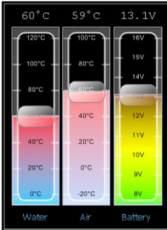
These 3 bars will indicate water and air temperatures and also the battery voltage as it is supplied to the ECU.
