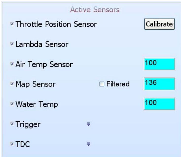
A screenshot of the 'Active Sensors' configuration window. It lists several sensors with checkboxes and numerical input fields. The 'Throttle Position Sensor' has a 'Calibrate' button. The 'Air Temp Sensor' has a value of 100. The 'Map Sensor' has a 'Filtered' checkbox and a value of 136. The 'Water Temp' has a value of 100. The 'Trigger' and 'TDC' sensors have dropdown arrows.
