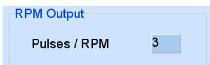
This block is for Rev counter calibration. You can adjust the number of pulses per revolution which is handy for engine conversions.
