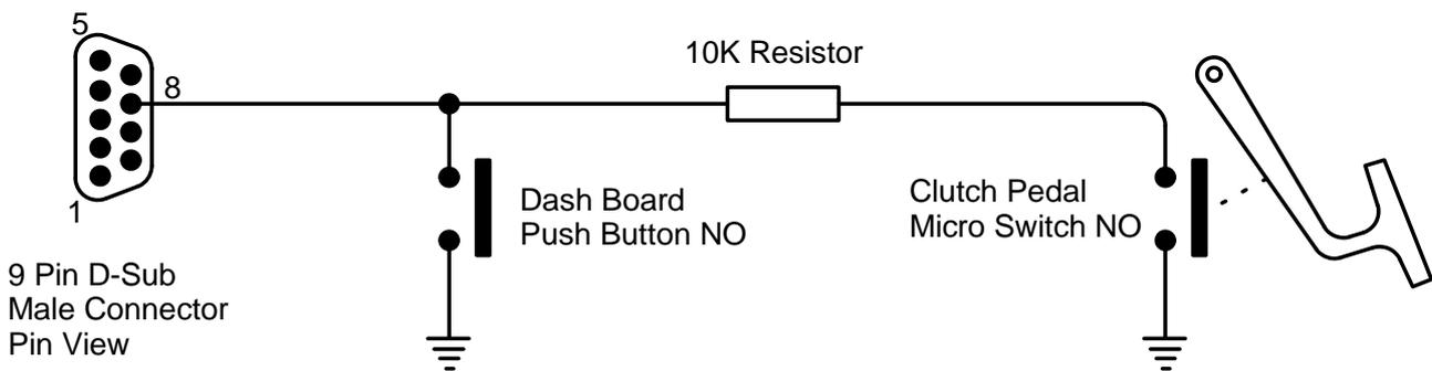
*Note: Pin 8 can also be connected with the PC interface cable for tuning while using the button.*
