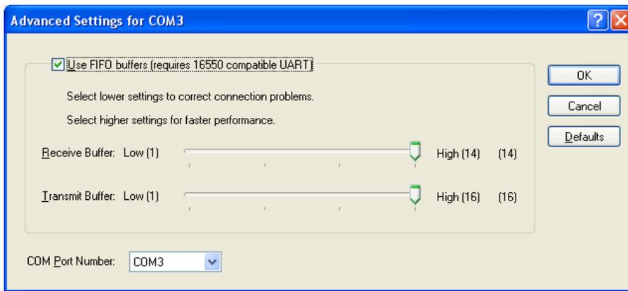
The settings for the USB cable must be the same as above. Note that the Com port must be Com 1 to 10. Higher numbers will not be detected.
