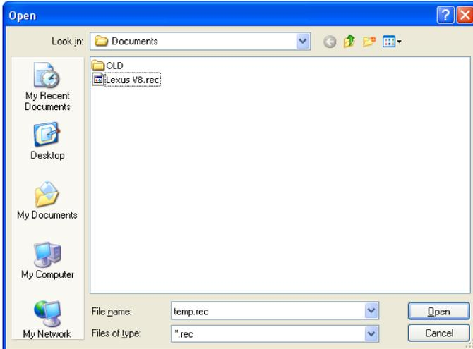
To do adjustments remotely first load in the engine map and then open the file. Play it back and do adjustment. Then save the Map file by pressing save from PC.
