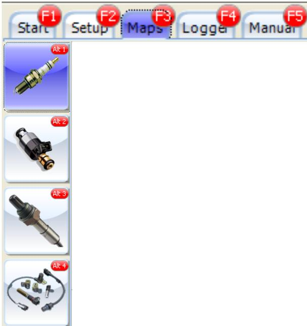
Click on the Maps tab to get information on the tuning maps of your engine. Startup Maps are being preset before the ECU has been shipped. These maps may require to be adjusted to suit your engine. Some maps for tuned engines are also supplied and may only require minor adjustments.
