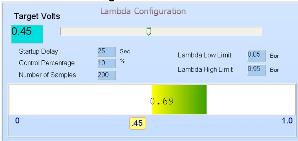
This block is used to set control parameters for the ECU to use the lambda signal to adjust fuel enrichment while driving. Note that lambda sensor correction will only operate when the engine temperature is above 60°C.
