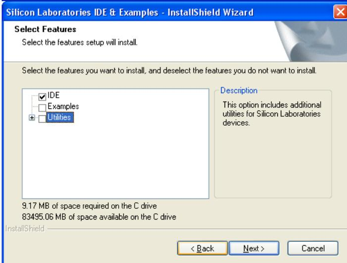
You will not need these and they will only take up unnecessary disk space. No harm if you install the complete programmer. Connect the USB programmer to the PC only and start the program at the start button, activate Silicone Laboratories and click on Silicone Laboratories IDE.
