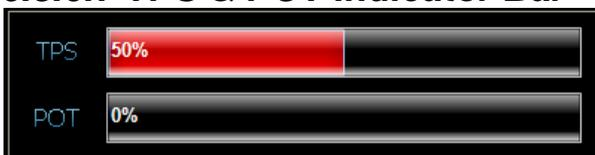
The TPS% bar indicates the throttle position at that stage. If it is calibrated, it will indicate from 0 to 100 % between closed and open throttle.
