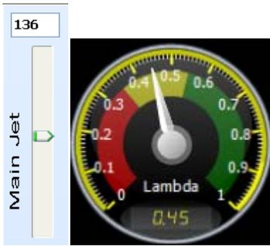
Remember this main jet value so that you always end with this value during tuning. The main jet slider is used during tuning to see if you are close to the right air-fuel mixture.
