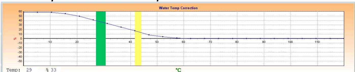
This map is to set the water temperature correction mostly for cold starting. The colder the engine is, the richer the mixture should be. Try and start your engine on a cold morning. Set the correction factor in the positive region of the map, by increasing fuel until the car starts. As the engine temperature increase, keep reducing the mix until it idles smoothly. Always adjust the setting on the right of the yellow bar. The hotter the engine becomes the less the factor will become, so your
