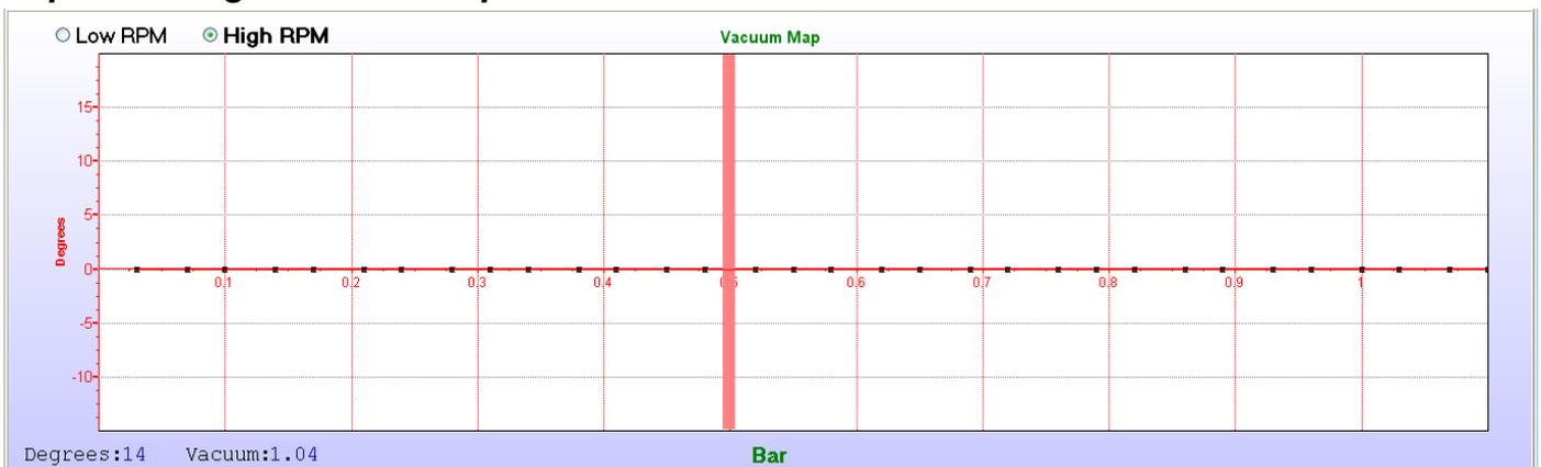
Set a basic RPM timing map to start at 8°BTDC degrees and idle at 15 to 17°BTDC degrees. Increase the timing from 1000RPM to 3500RPM up to 32°BTDC. Keep it flat till maximum timing.
