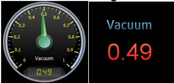
VACUUM - This is the vacuum value from the MAP sensor. It is measured from Absolute vacuum to atmosphere and also boost pressure for Turbo engines. Double click will toggle between the two options.
