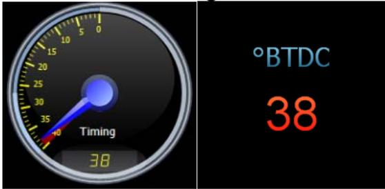
TIMING - This is the calculated timing of all the timing maps and will be the same as seen on the timing light. Double click will toggle between the two options.
