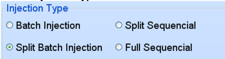
**Injection Type** – This setting is an indication of what type of fuel injection setup the ECU was programmed for. On some models this may be adjustable depending on the firmware.
