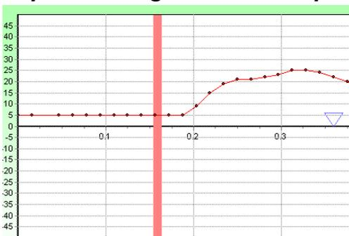
If it is an automatic car put it in drive and do the following two adjustments. Then if it has an air conditioner, switch it on and repeat the steps while in drive. A Manual car only requires one step. Now see where the vacuum bar stabilize and adjust a step in the graph to add about 4 degrees of timing.
