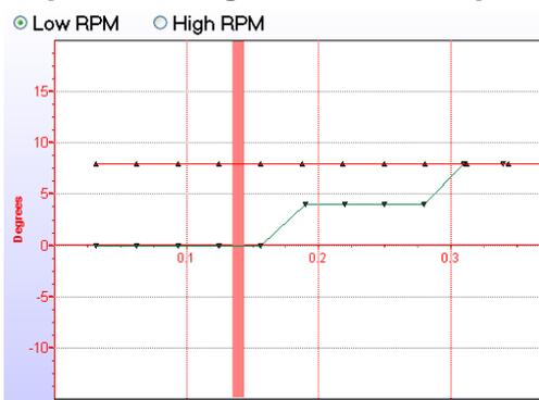
Also make sure that the Fuel Map Vacuum correction is on a flat graph during idling as with timing. If the engine hunts it is most probably a lean mixture at the Idle Jet.
