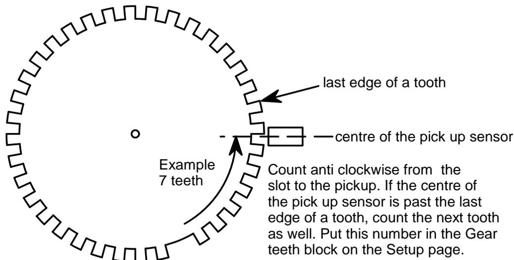
The trigger point of the sensor is the centre of the sensor to the last edge of the tooth or trigger plate (Trigger Edge 0°). On a 36-1 gear the pitch is 10 degrees. To adjust the Timing BTDC block you can guess a setting for the centre of the pickup between the trigger edges of the adjacent teeth. See the sketch below. When the engine is running, adjust it till the software correlates with the timing light.
