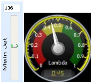
Now stop and punt the gearbox in neutral. Let the engine idle and adjust the idle jet till the engine run at just higher than Stoich or 0.45Volt. If you decrease the idle jet by 3 increments the engine should go lean and start to labor. Use the D & C keys for 1 increment or the F & V keys for 10 increments.
