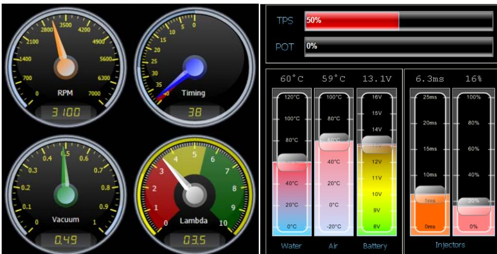
This block displays the current analogue data as it is measured by the ECU for while the engine is off or running. These values are used to set and tune the ECU correctly for all conditions.
