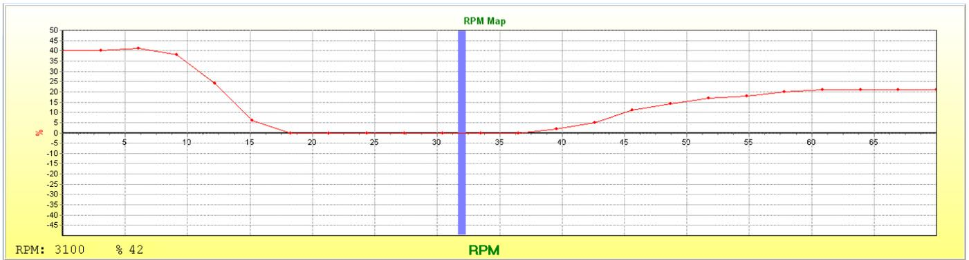
The ECU will now control on different air-fuel ratio's to let the engine run from rich to lean.
