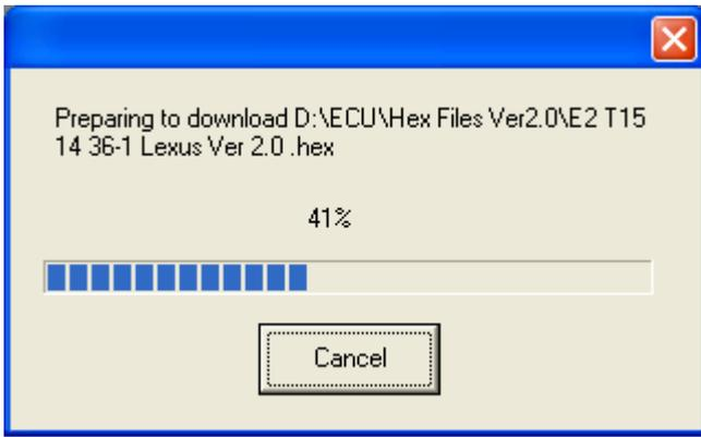
Click the disconnect
