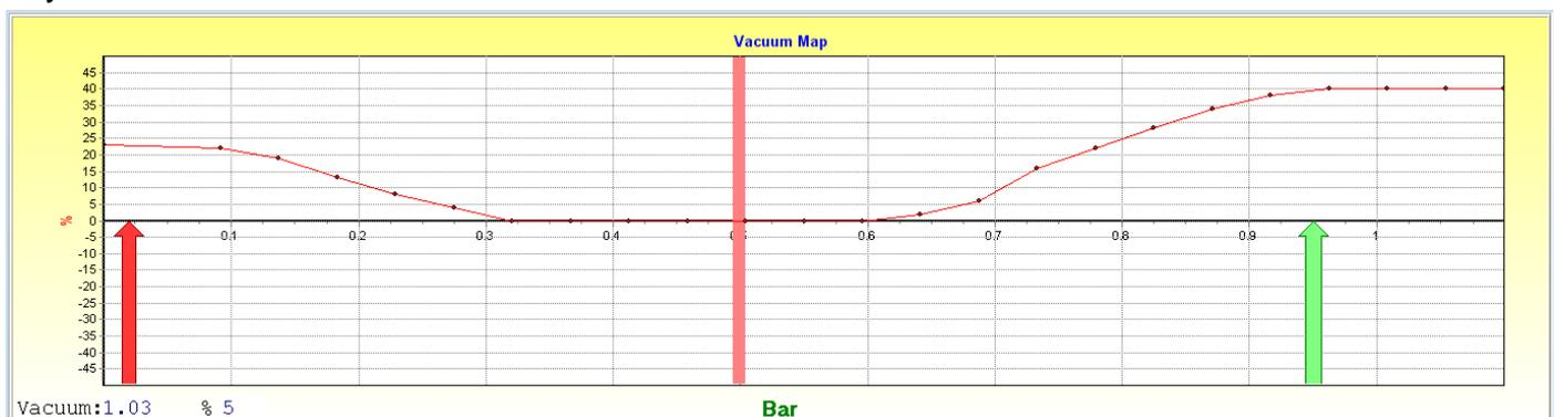
Now keep the load in the middle of the graph and adjust the bottom RPM map at different RPM's to achieve the correct mixture.
