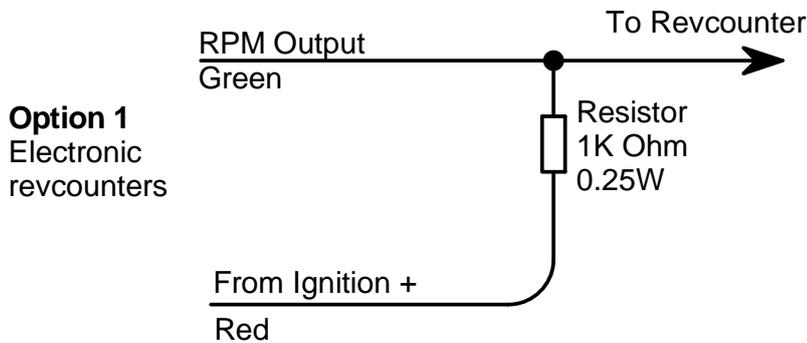
Coil Negative Rev Counters may not work with the above connection because they require a spike rather than a ground signal. In this case the rev counter must be connected to coil negative. Then you will have to calibrate the rev counter or try the circuit below. This circuit will generate a spike for the rev counter and will work in most cases. If it still does not work try a 220 Ohm 5 watt resistor instead.
