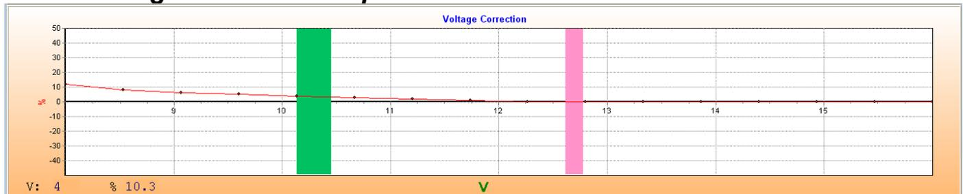
This map is used to set battery voltage compensation to enrich the fuel mix as battery voltage decreases during cranking. The lower your alternator and/or battery voltage is, the less fuel gets injected into your engine, causing it to run lean. Increase the percentage to compensate for a lean condition. A high voltage will require the least amount of fuel.
