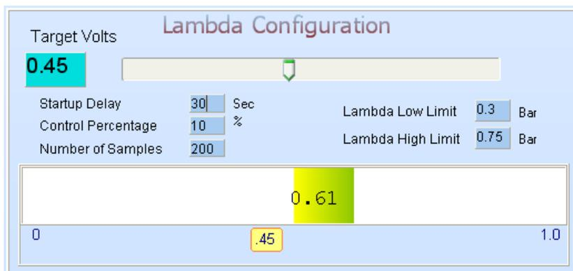
Start with the middle RPM's at 3200 and then adjust the top Vacuum graph at different loads with the throttle. Keep in mind what the air-fuel ratio should be for the different loads. Adjust the graph till you achieve the correct mixture.
