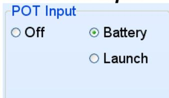
The Pot Input can be used for one of the following. Battery input or use as a launce control. For a normal car, set it to battery so that battery voltage compensation can be adjusted. If any other function is selected, a fixed battery voltage of 12.7 volt is forced into the ECU. For racing cars you can use the launce control function. See [Launch Control](#) on how to use the launce buttons.
