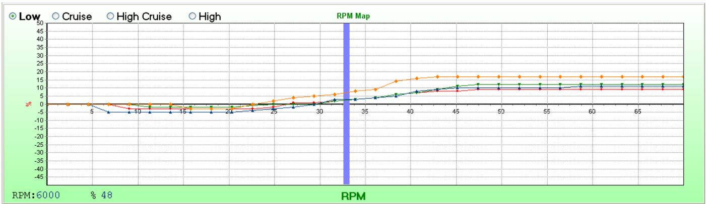
Set main jet slider till the lambda reaches 0,45Volt which is Stoich or lambda 1. This will ensure that the graphs are evenly spaced over the zero line. You can press the Q & A keys for 1 increment or the W & S keys for 10 increments.
