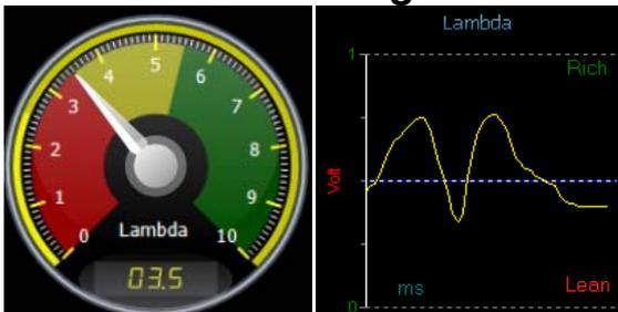
LAMBDA - This is the Lambda value read from the Oxygen sensor. It is measured in volts from 0 to 1 Volt. Where 0 Volt is lean, 0.45 Volt is Stoichiometric or 14.7 air-fuel ratio and 1 Volt is rich. Double click will toggle between the two options.
