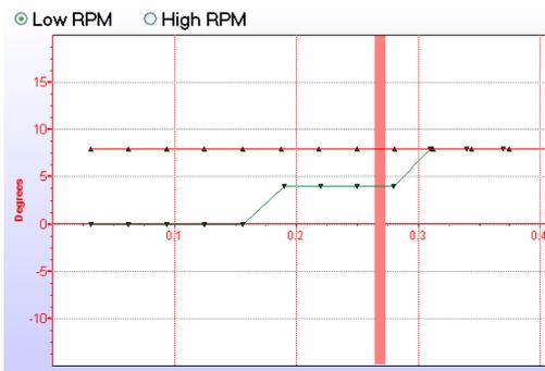
Adjust the dots on the Fuel vacuum graph to achieve a air fuel ratio the same as for no load idling. These setting will let the engine idle stronger when more power is used for automatic transmissions and air conditioners or power steering.
