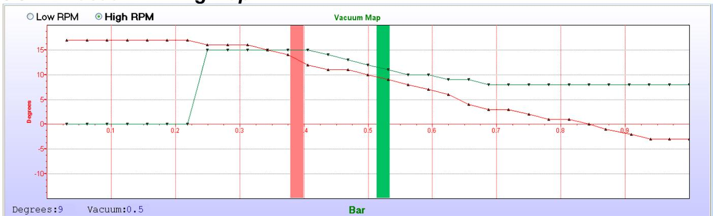
On this map you can set the amount of ignition advance and retard for a specific vacuum or boost pressure value. There are 2 maps with 32 divisions for the map sensor which can be adjusted from -15° to +20° in 1° intervals.
